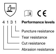
Pictogram and performance levels according to EN 388:2003 (highest performance level: 4/cut resistance: 5)
