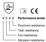
Pictogram and performance levels according to EN 388:2003 (highest performance level: 4/cut resistance: 5)
